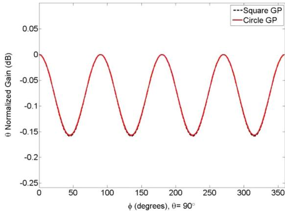
Fig. 10. 800 MHz antenna pattern comparison on a square and circular ground plane.
