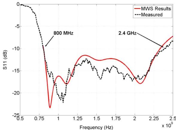
Fig. 15. Comparison of  $S_{11}$  of calculated and measured antenna.
