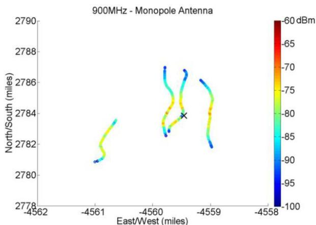
Fig. 22. Power level received when a 900 MHz, 2.1 dBi monopole is used at the ground station indicated by an “X”.
