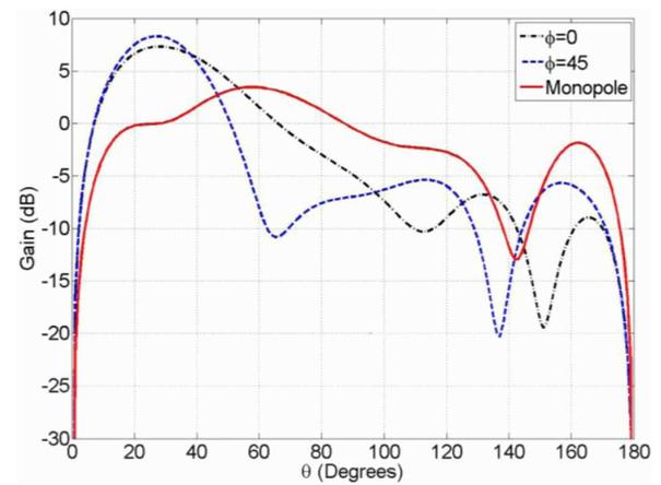
Fig. 17. STHMA  $\theta$  gain (dBi) at 2.3 GHz compared to the gain of a resonant monopole (2.3 GHz) at  $\phi = 0^\circ$  and  $45^\circ$ ,  $\theta = 0 : 180^\circ$ .
