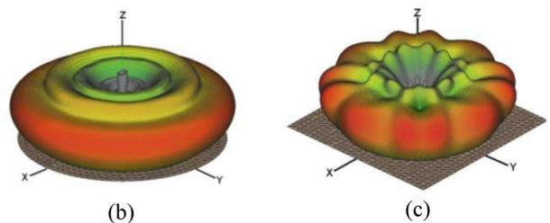
Fig. 7. The antenna pattern of a monopole modeled in FEKO over (a) infinite (b) finite circular (c) finite square ground plane.
