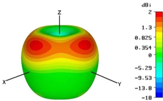
Fig. 18. 3D radiation pattern of STHMA at 800 MHz.
