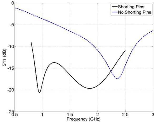
Fig. 3.  $S_{11}$  of the initial antenna design with and without shorting pins.
