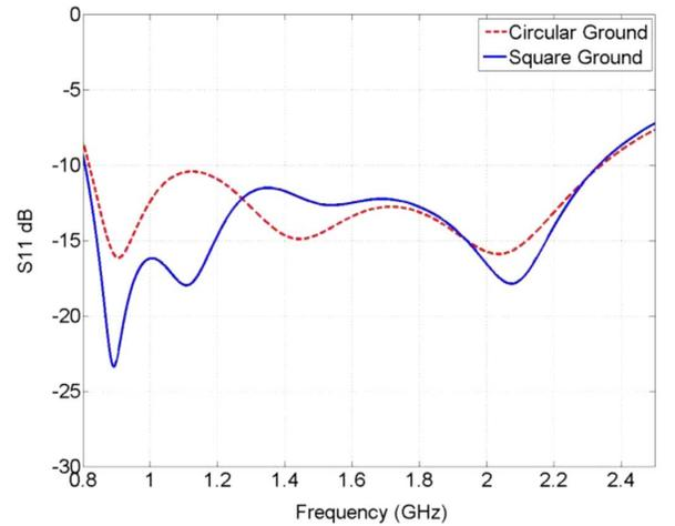
Fig. 12. Calculated  $S_{11}$  comparison using a square ground plane and a circular ground plane.
