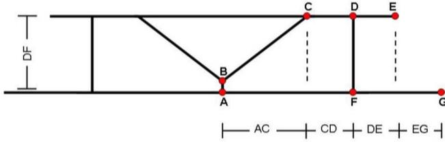
Fig. 8. The proposed antenna design showing variables used during optimization. Optimized line segment lengths:  $DF = 25.4$ ,  $AC = 45.77$ ,  $CD = 19.43$ ,  $DE = 3.14$ , and  $AG = 126.63$  mm.
