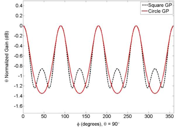
Fig. 11. 2.4 GHz antenna pattern comparison on a square and circular ground plane.
