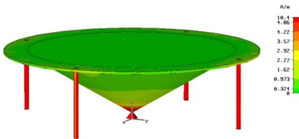
Fig. 4. Maximum surface current at 1 GHz—Infinite ground plane prototype.
