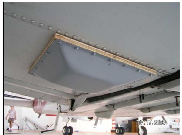
Fig. 21. STHMA mounted on the belly of a Cherokee Airplane.
