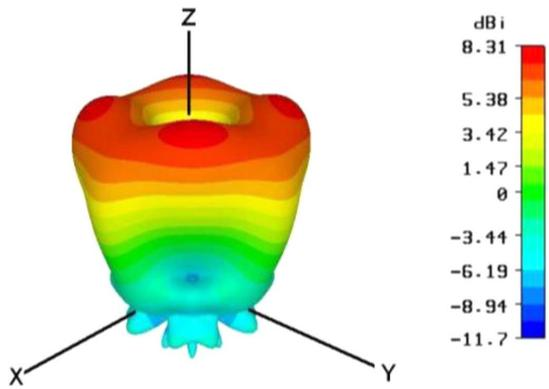
Fig. 19. 3D radiation pattern of STHMA at 2.4 GHz.
