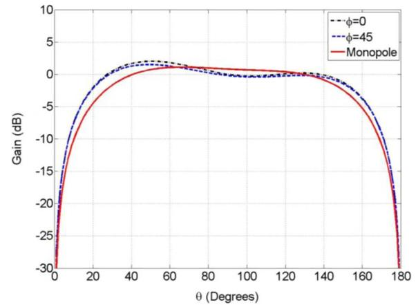
Fig. 16. STHMA  $\theta$  gain (dBi) at 800 MHz compared to the gain of a resonant monopole (800 MHz) at  $\phi = 0^\circ$  and  $45^\circ$ ,  $\theta = 0 : 180^\circ$ .
