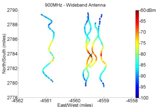
Fig. 23. Power level received at 900 MHz when the STHMA is used at the ground station indicated by an “X”.
