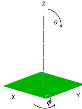
Fig. 6. A monopole antenna modeled in FEKO over an infinite ground plane.
