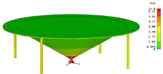
Fig. 5. Maximum surface current at 2 GHz—Infinite ground plane prototype.
