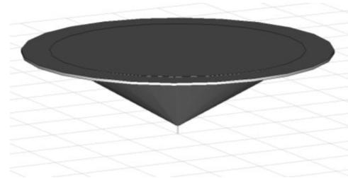
Fig. 1. An optimized design on an infinite ground plane without shorting pins.
