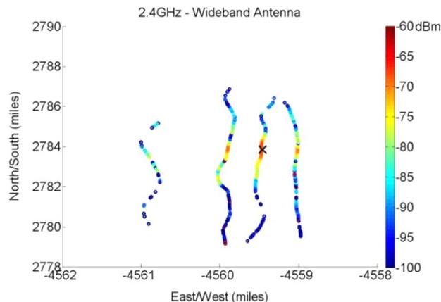
Fig. 25. Power level received at 2.4 GHz when the STHMA is used at the ground station indicated by an ‘X’.
