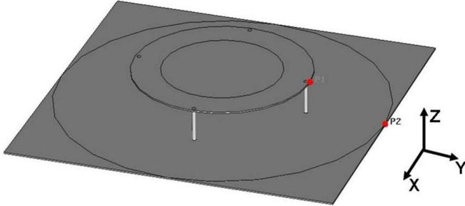
Fig. 9. A three dimensional view of the STHMA on a square ground plane modeled in MWS.
