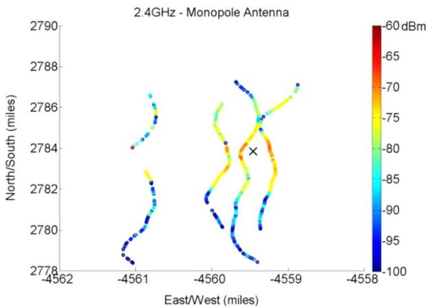
Fig. 24. Power level received when a 2.4 GHz, 2.1 dBi monopole is used at the ground station indicated by an “X”.
