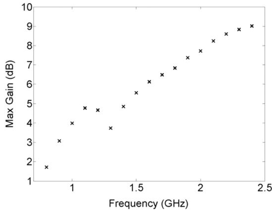
Fig. 13. Maximum gain (dBi) versus frequency of the STHMA.
