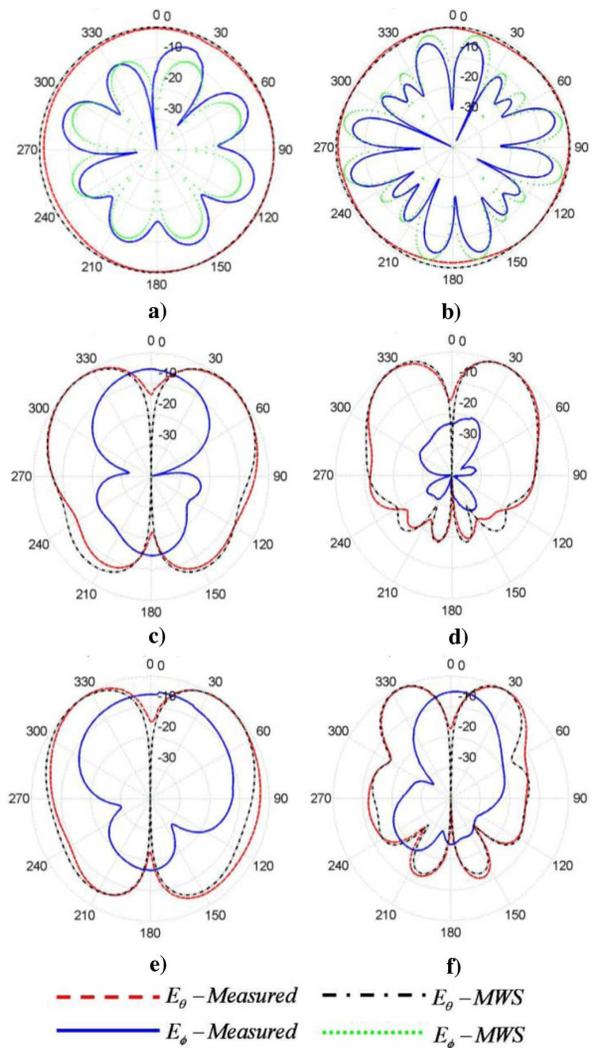
Fig. 20. STHMA normalized 2D radiation pattern measurements and comparison to MWS. (a) 1.0 GHz,  $\phi$  0:360,  $\theta$  90, (b) 2.4 GHz,  $\phi$  0:360,  $\theta$  90, (c) 1.0 GHz,  $\phi$  0,  $\theta$  0:360, (d) 2.4 GHz,  $\phi$  0,  $\theta$  0:360, (e) 1.0 GHz,  $\phi$  45,  $\theta$  0:360, (f) 2.4 GHz,  $\phi$  45,  $\theta$  0:360.
